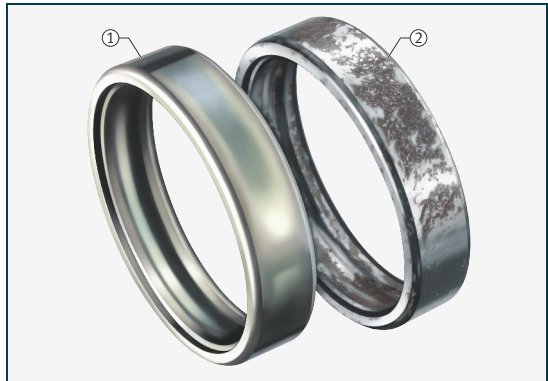
Figure 39 Bearing rings after 24 h on a test rig in the salt spray test
