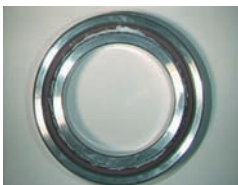
Photo. 6.1 Filling grease into angular contact ball bearing
