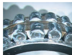
Photo. 6.2 Filling grease into cylindrical roller bearing
