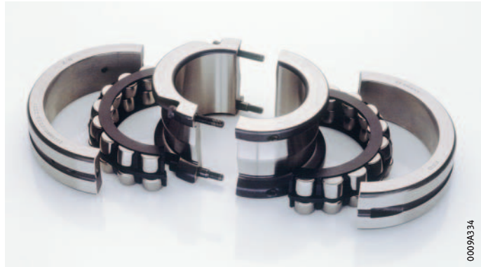
Figure 9 Split spherical roller bearing with split solid cage made from glass fibre reinforced polyamide or brass, with integral locking rings
